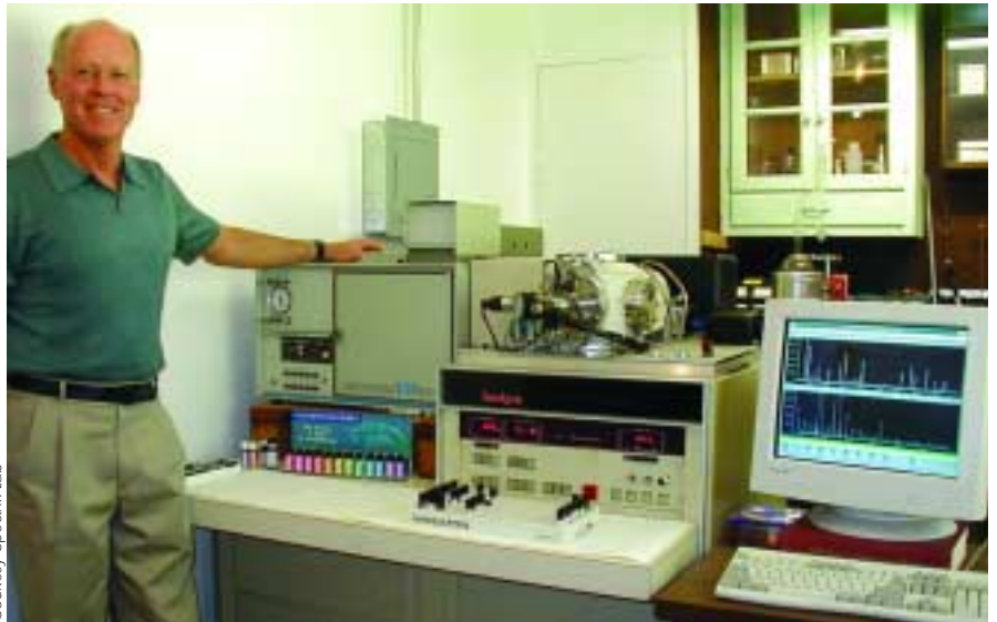
Larry Jones, owner of Spectrix Lab in Santa Cruz, California, says the Gas Chromatograph-Mass Spectrometer (GC/MS) is science's most powerful research tool for analyzing essential oils.
